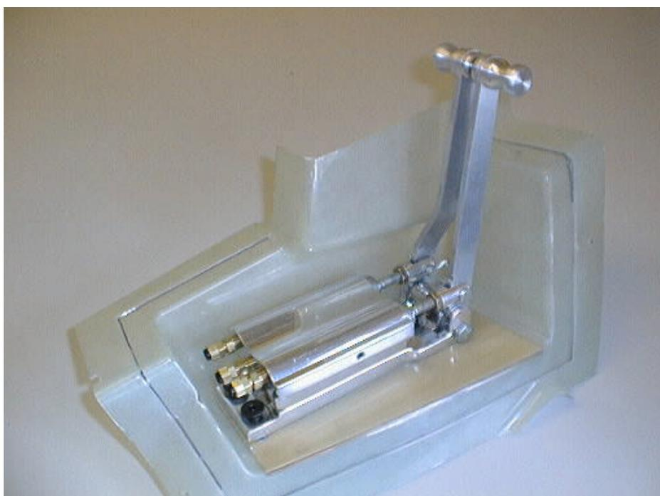
*Fig 7. Platform / master cylinder sub-assembly.*
