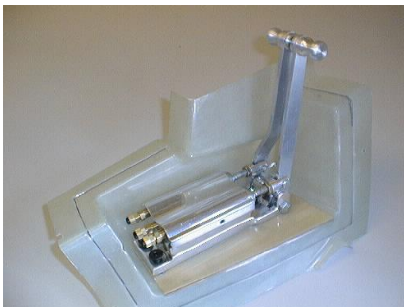
Fig 7. Platform / master cylinder sub-assembly.
