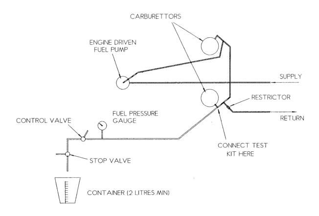
Arrangement of test equipment for fuel flow check.
