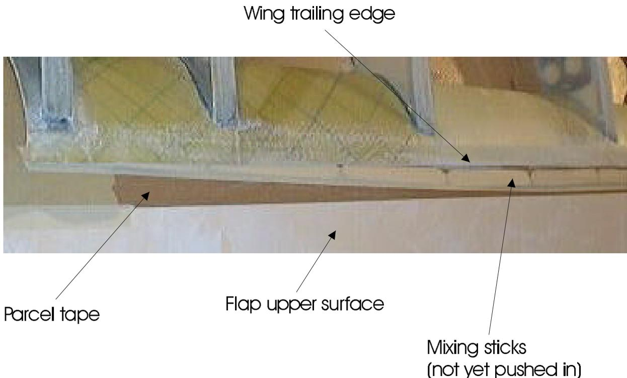
Fig 24. Mixing stick spacer arrangement.
