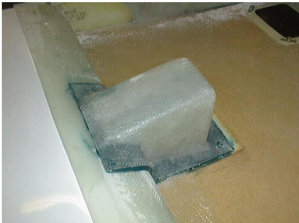
*Fig 22. Aileron mass balance box bonded into place.*
