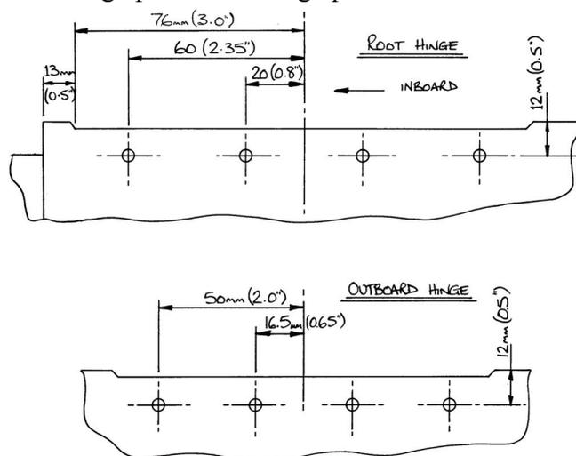
Fig 2. Underside of wing showing hinge screw centres.
