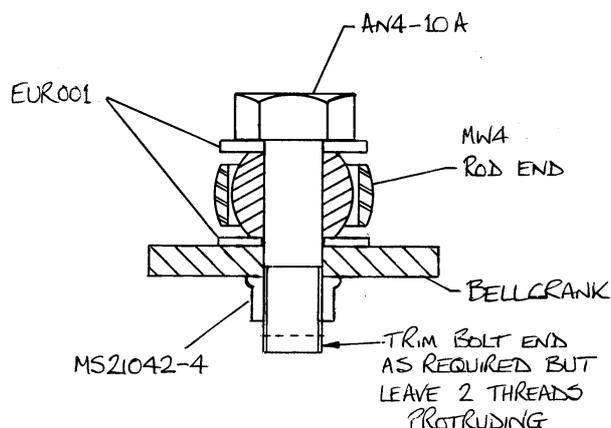
Fig 5. Typical attachment of rod-end to a bellcrank.
