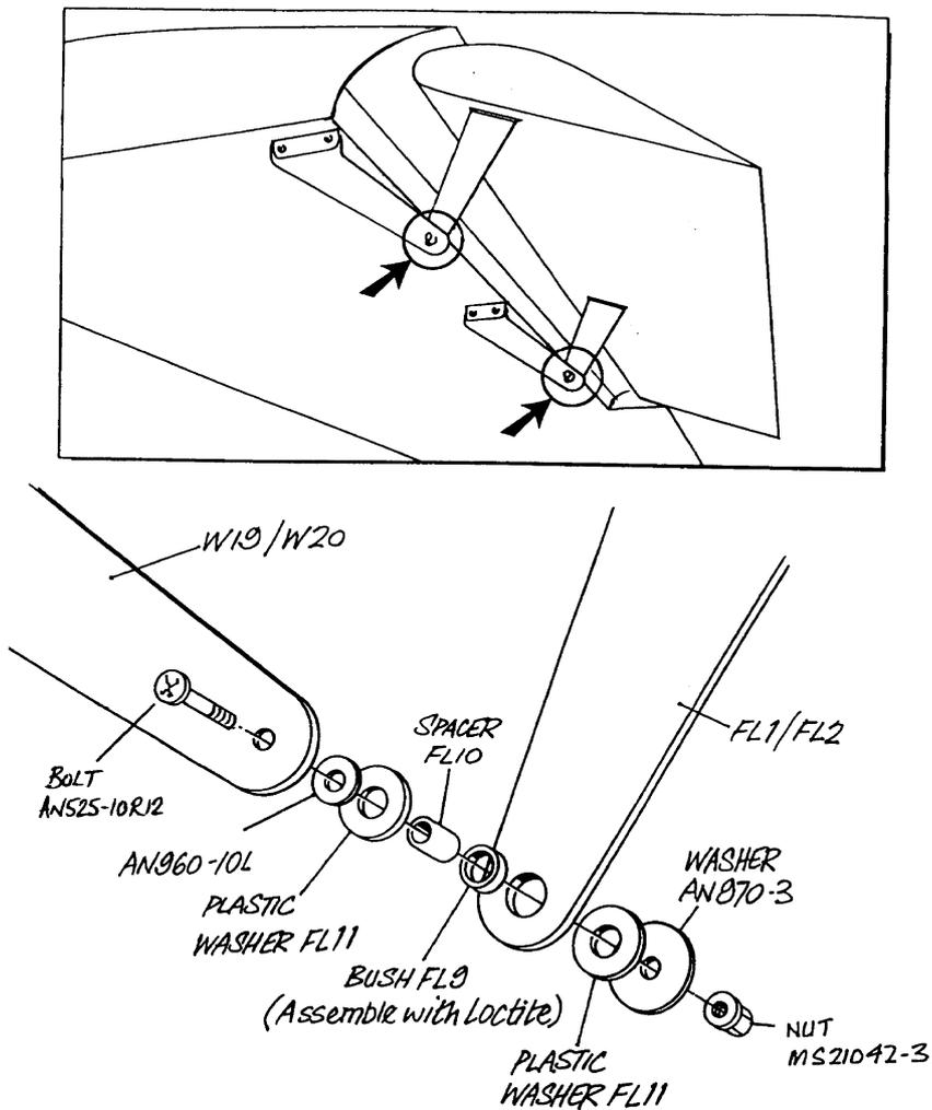
Fig 21. Inboard and mid flap hinge arrangement.
