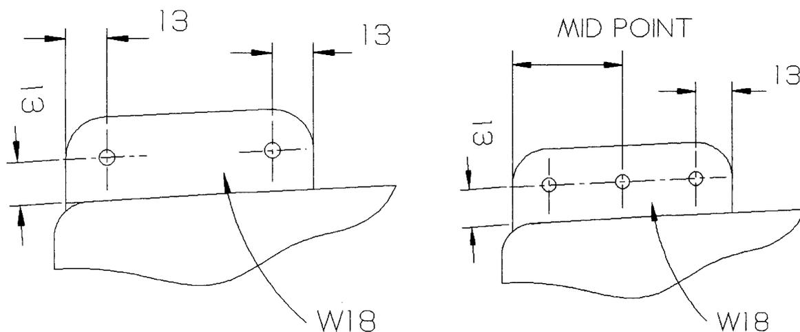
Fig 10. Hole centres (inboard and mid hinge connectors). Fig 11. Hole centred (outboard hinge connectors).
