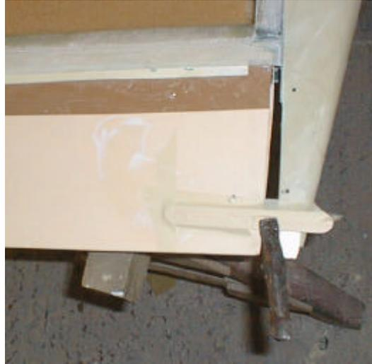
Fig 23. Aileron clamped in neutral.
