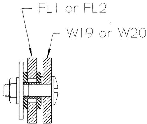
*Fig 7. Section through inboard and mid flap hinges.*
