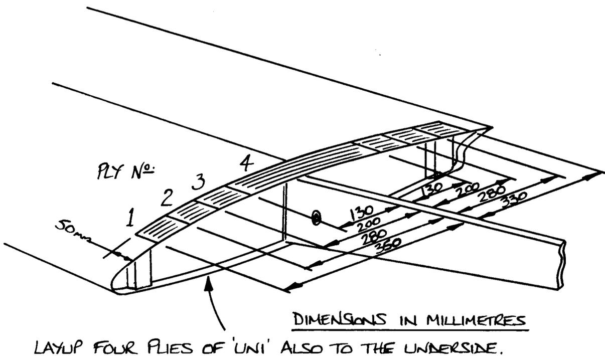
Fig 26. 'Uni' plies at wing root.
