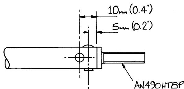
Fig 4. Rivet hole positions in ½" dia. push-rod.
