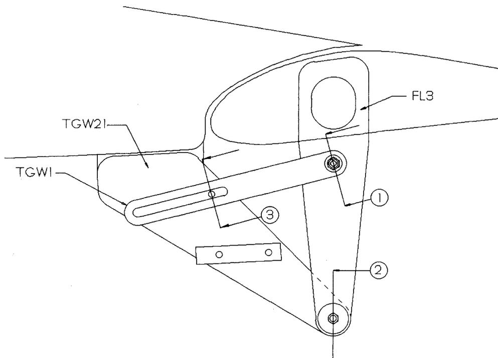
*Fig 14. Outboard flap hinge with section locations.*
