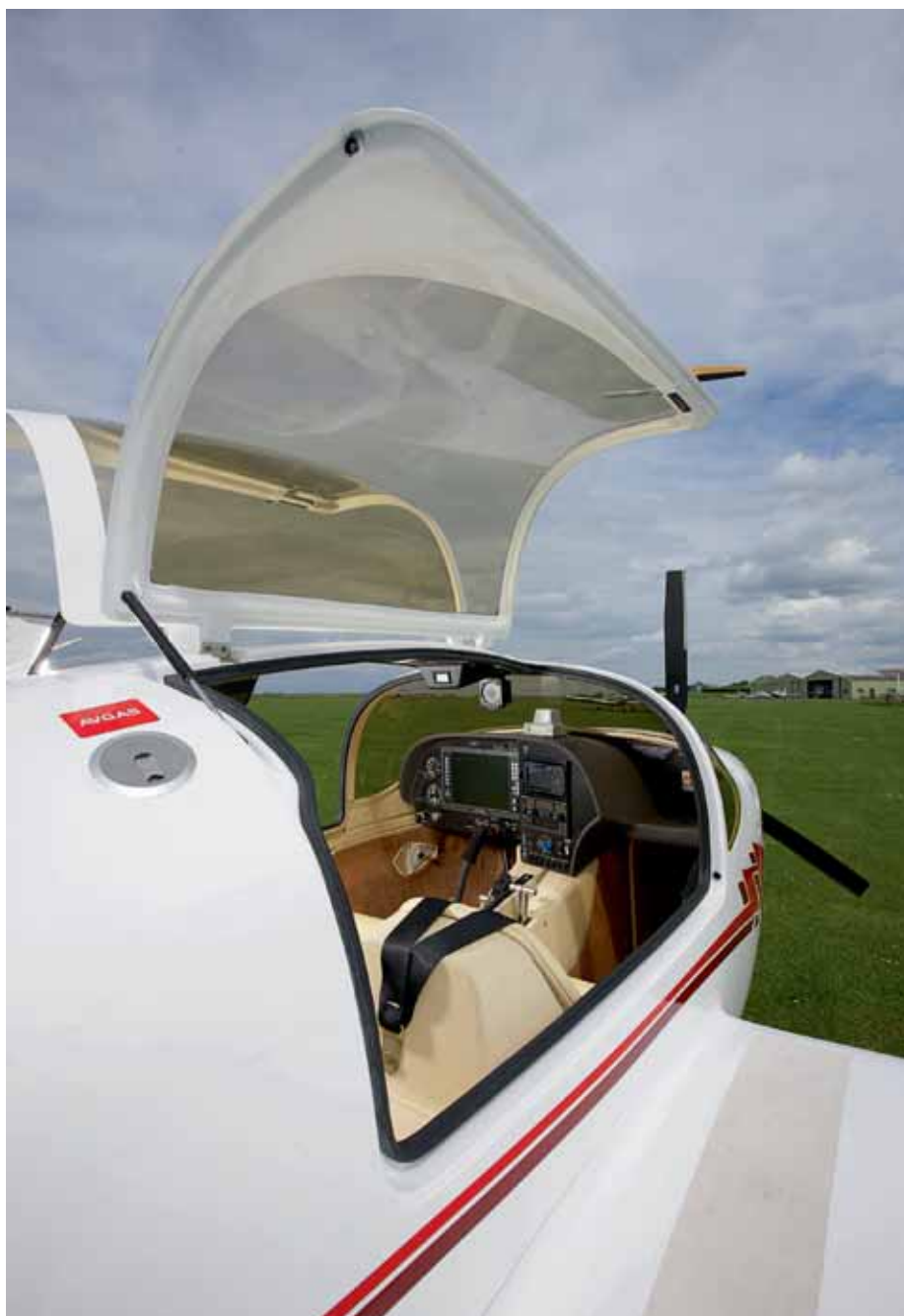
Gull-wing doors make getting into and out of the Europa simple. Note big windows for great visibility.
