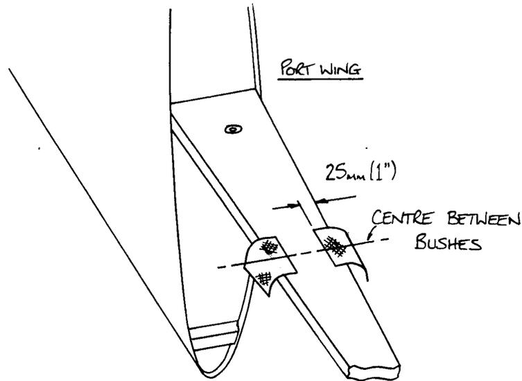
*Fig 13. Bracket plies in position on port spar.*
