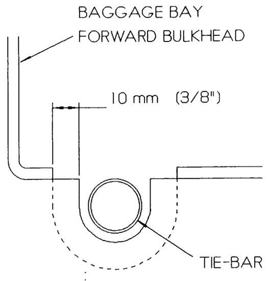
*Fig 10. Section through baggage bay centre tunnel.*
