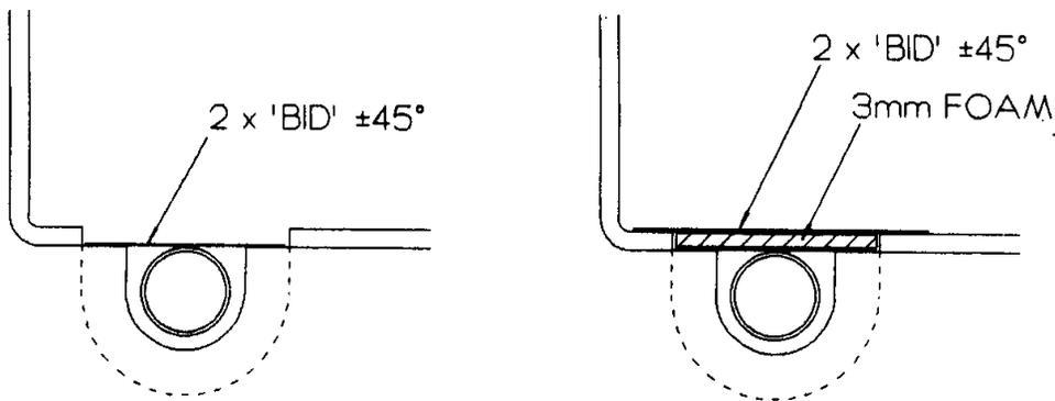
Fig 11. Section through tunnel detailing layup sequence.
