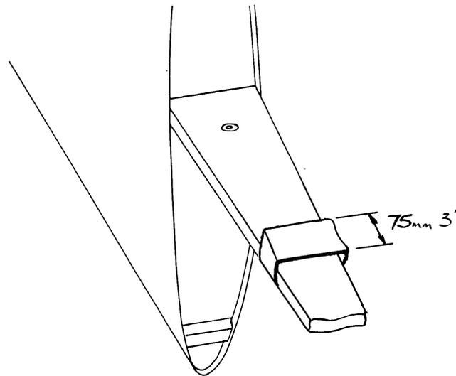
Fig 15. Spar strap trimmed to size
