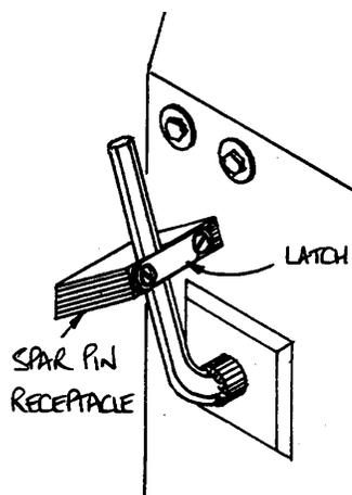
The safety latch on the port side where the pip-pin is used can be removed altogether.
