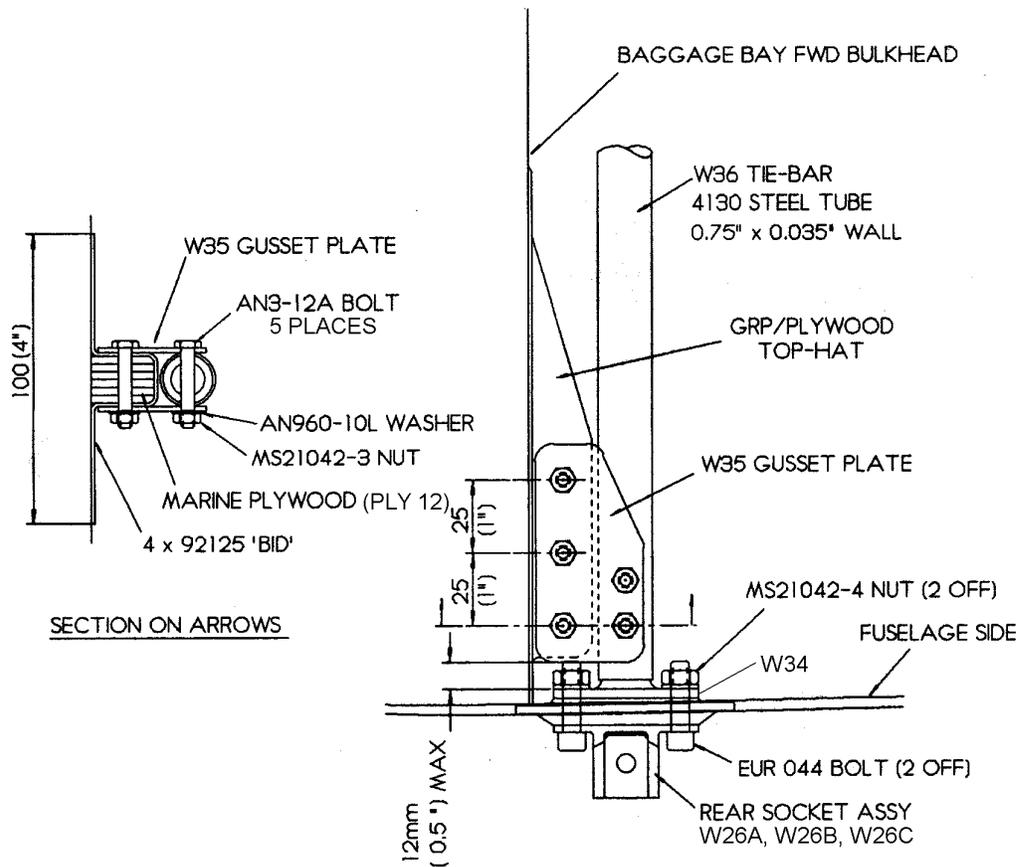
Fig 8. Top and sectional view of tie-bar and socket (port side).
