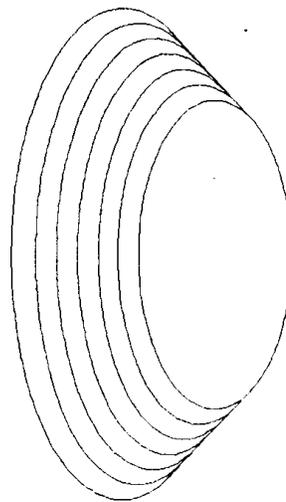
*Fig 7. Plywood mounting pad.*
