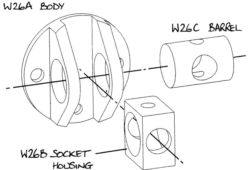
Slide the barrel in to the assembly from one side and rotate it so that the large and small holes align with the holes in the housing. Check that your 1/4" diameter BLS4R11N pip-pin will pass through the small hole without hindrance. A check with the pip-pin including the new W24/5 wing pin would also be sensible at this stage.
