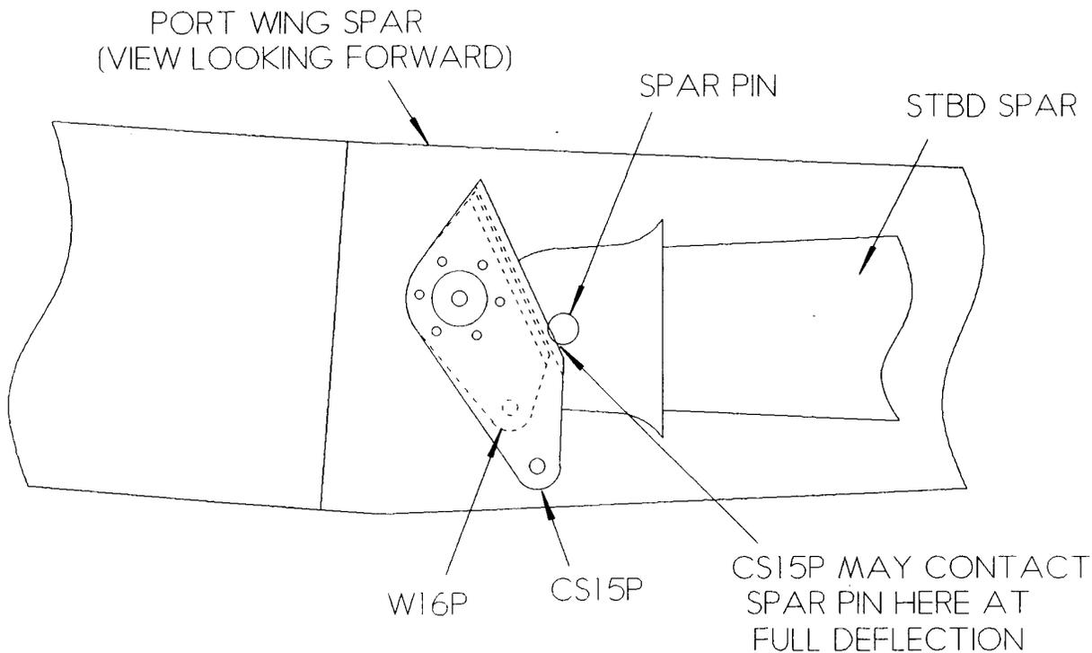
To avoid contact with the pin, the corner of CS15P should be removed as shown in figure 5. Ensure that the inner corner is radiused as shown.
